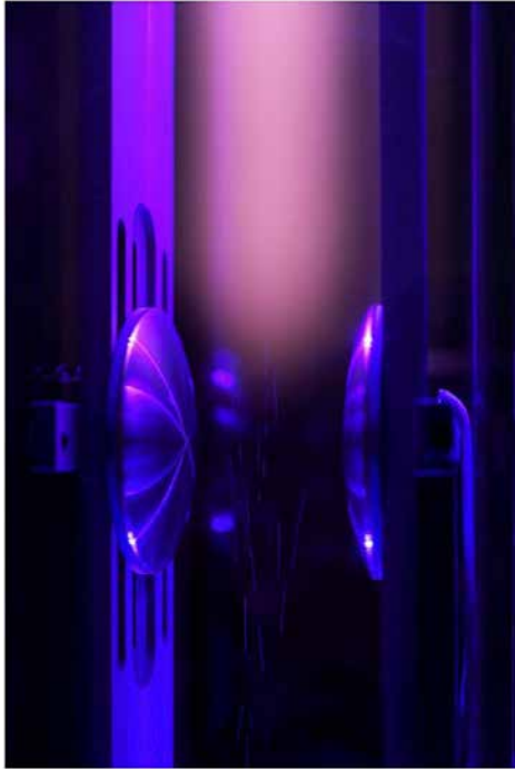
Figure 7. Dust particles falling in a plasma afterglow. The electrodes on the sides induce a static electrical field, which allows the study of charging, de-charging and drift of dust particles. This knowledge is used for the prediction of particle behavior in lithography-related plasmas. Photo: Eindhoven University of Technology. Reproduced with the permission of Bart van Overbeeke Fotografie.
