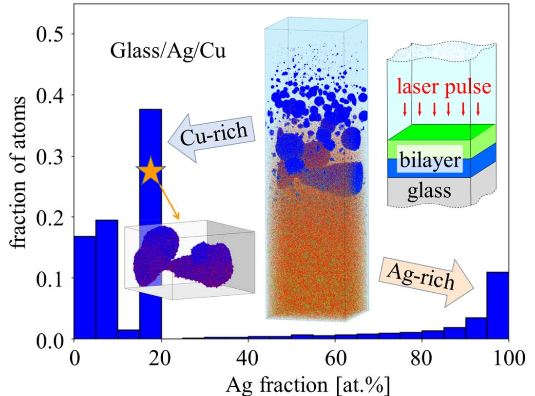
Explained by complex dynamic interaction between the ablation plume and liquid environment: Accumulation of plume at the interface with liquid → formation and decomposition of a hot liquid layer that prevents mixing and yields large nanoparticles
