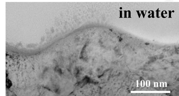
Surface features produced by single shot ablation of Cr (001) target irradiated at  $6000 \text{ J/m}^2$  incident laser fluence in air and water
