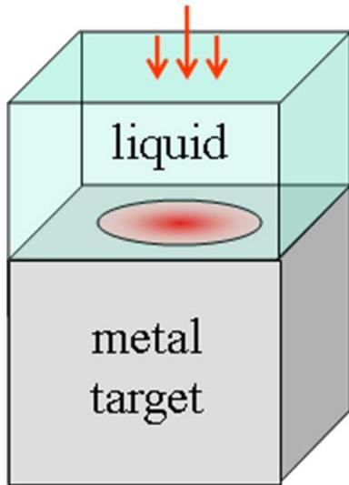
surface micro/nano-structuring by laser processing in liquids
