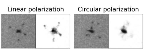
Shadowgraphs that were made during the experiments demonstrate formation of cross-like structures as a result of droplet break up. We observe formation of jets along the line of laser pulse and also in the perpendicular plane. Crossshape jets are observed in our experiments only for linearly polarized laser pulse. For non-polarized laser pulse direction and number of jets can be different for different experiments.
