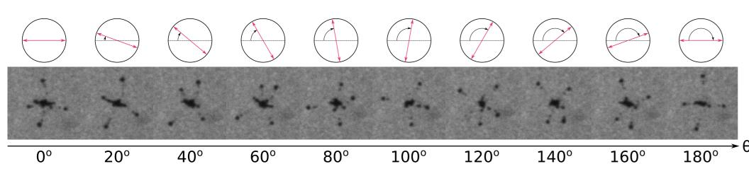
By rotating the half-waveplate we can rotate the polarization plane of the laser radiation. The snapshots of the fragmented droplet taken at the same moment of time for different polarization plane orientation demonstrate that jets are guided by the rotation of the laser polarization plane. Moreover, the jets directions in the experiments are correlated with the direction of the laser radiation electric field vector E.
