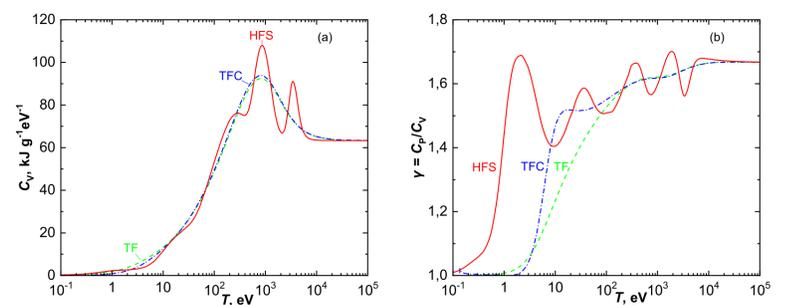
**Figure 3:** (a) Electron heat capacity at constant volume  $C_V$  and (b) adiabatic index  $\gamma = C_P/C_V$  as functions of the temperature  $T$  for Mo at constant density  $\rho = 10.22$  g/cm<sup>3</sup> according to different models: green dashed curves—TF; blue dash-dot curves—TFC; red solid curves—HFS [3].
