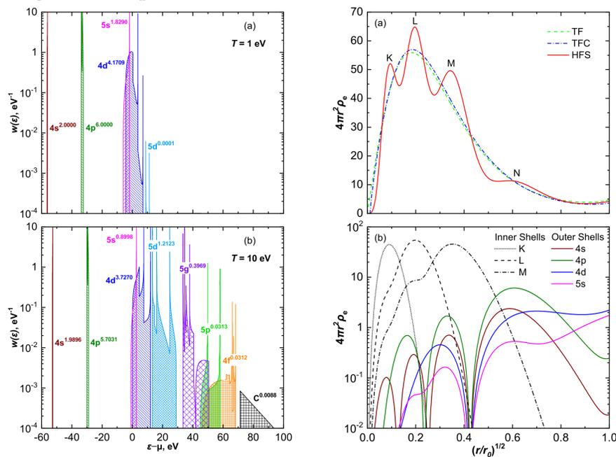
**Figure 1:** The density of states for outer electron shells of Mo ( $\rho = 10.22$  g/cm<sup>3</sup>) at temperatures (a)  $T = 1$  eV (here the chemical potential  $\mu = 1.3587$  eV) and (b)  $T = 10$  eV ( $\mu = -1.6297$  eV) calculated in the framework of the HFS model [3].
