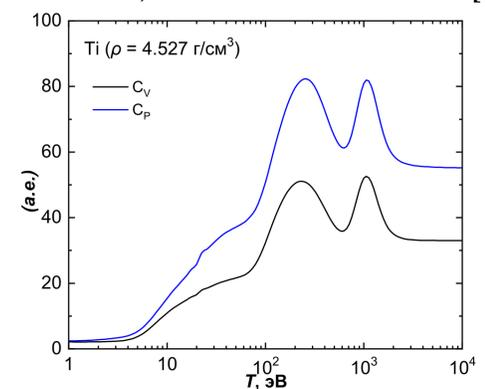
**Figure 4:** Electron heat capacity at constant volume  $C_V$  and pressure  $C_P$  as functions of the temperature  $T$  for Ti at constant density  $\rho = 4.527$  g/cm<sup>3</sup> according to HFS model.
