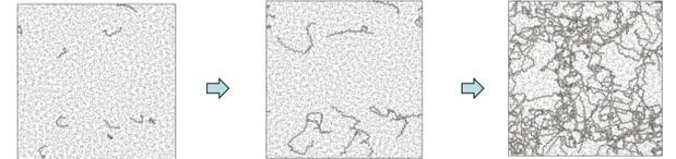
Figure 2. The scheme of the polymer matrix preparation using "radical-like" polymerization (M. Perez et al. J. Chem. Phys. 128, 234904 (2008))
