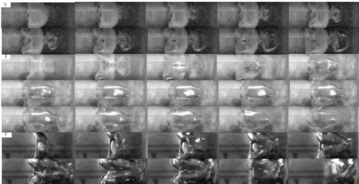
**Fig. 7. Images of bubble collapse at  $\gamma \approx 3$ . The 1<sup>st</sup> and 2<sup>nd</sup> rows: the strength of the pressure wave is 195 kPa; 3<sup>rd</sup> to 6<sup>th</sup> rows: the strength of the pressure wave is 265 kPa; 7<sup>th</sup> and 8<sup>th</sup> rows: the strength of the pressure wave is 550 kPa (the counter jet is indicated by an arrow). The time interval between images is 1/2000 second.**
