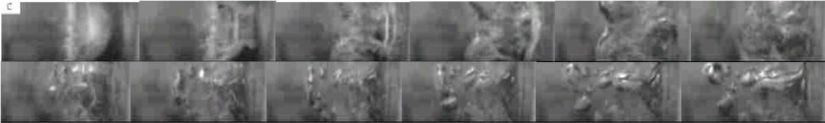
**Fig. 6. Images of bubble collapse flow at  $\gamma \approx 2$ . The strength of the pressure wave is 475 kPa. The time interval between images is 1/2000 second.**
