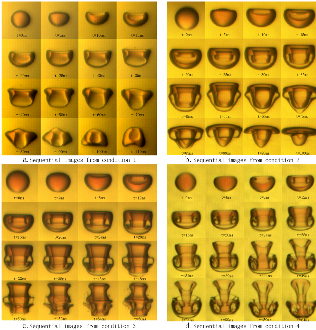
Fig. 4. A sequence of images from the experiments with the test conditions as Table 1. t=0ms is the beginning of the tank impacting at the stopper.
