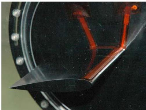
**Fig. 1. DBD plasma actuator installed at the wing leading edge**
