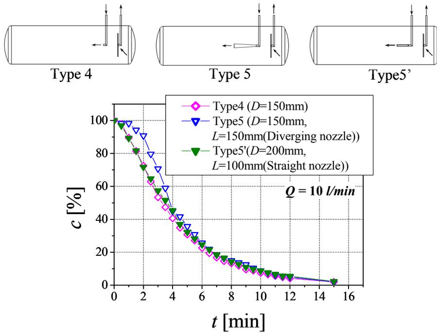
Fig. 10. Variation of concentration of drained water with time (Types 4, 5, and 5')
