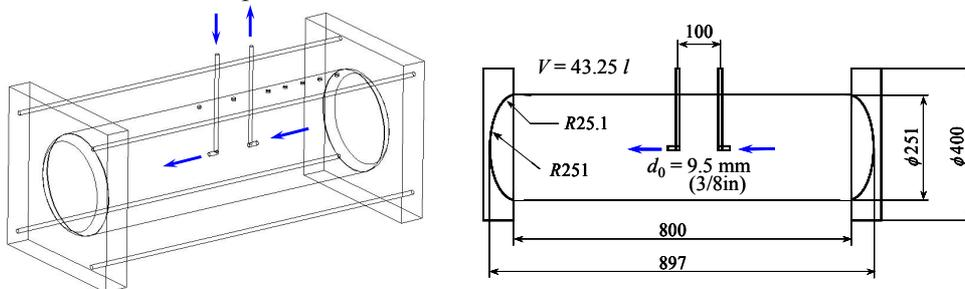
Fig. 2. Cylindrical tank
