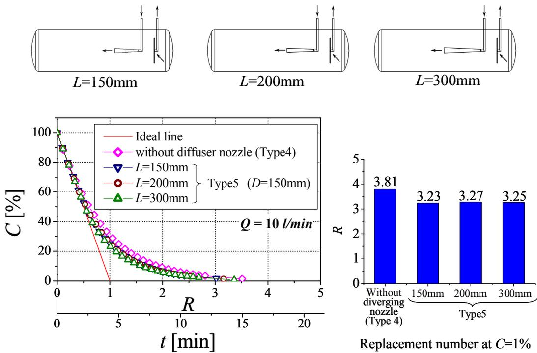
The variation of the concentration of drained water with respect to time is shown in Fig. 10. For the Type 5 tank, which has a baffle plate with  $D = 150$  mm and a diverging nozzle with  $L = 150$  mm, the concentration of drained water is higher than that for the other tanks until 6 minutes passes. The entrainment of old water to the jet of new water appears to have decreased as a result of the diverging nozzle.
