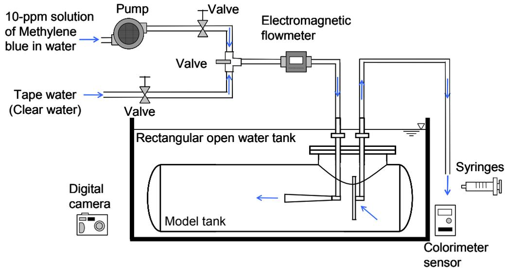
**Fig. 3. Schematic diagram of the experimental apparatus**
