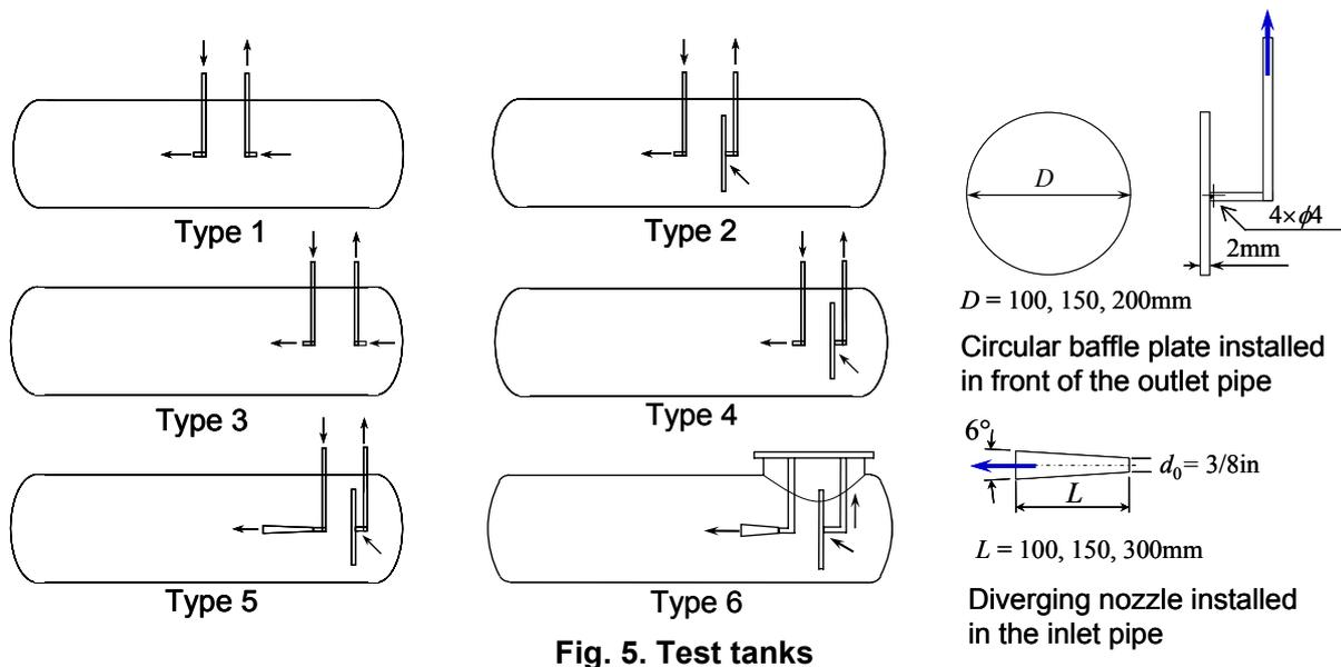
Fig. 5. Test tanks
