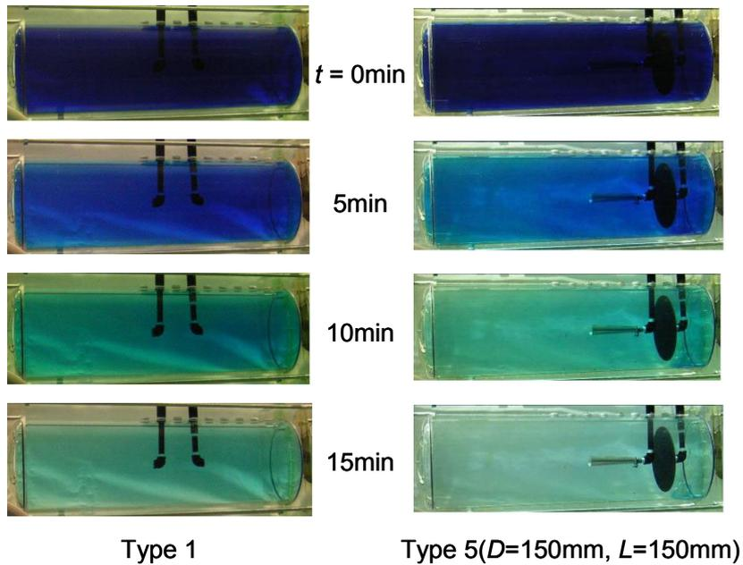
Fig. 11. Flow visualization in the tank (Types 1 and 5)
