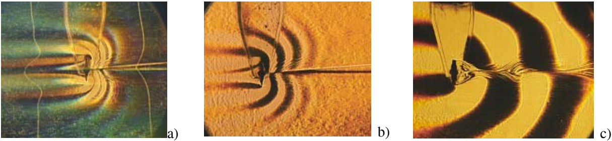
Fig. 4. Pattern of flow around a vertical strip with H_c = 2.5 cm moving from right to left: a, b) – T_b = 12.5 s, U = 0.1 cm/s; “slit-thread” and “slit-knife” methods; c) – T_b = 17.4 s, U = 0.3 cm/s, “slit-knife” method.
