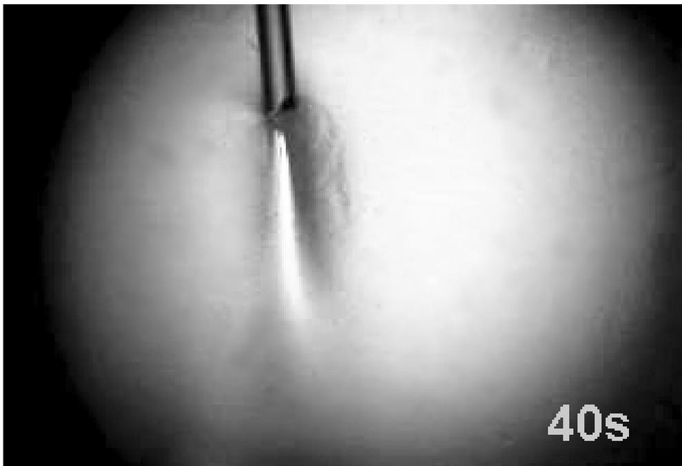
**Fig.1.Shadowgraph of the flow observed in zone of laser irradiation of gel. (Teopler's scheme. At the up of picture, it is seen the 600  $\mu\text{m}$  fiber of laser delivery system).**
