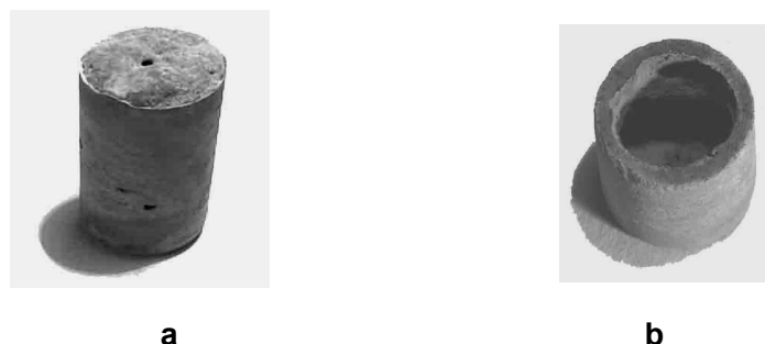
Fig. 1 Hollow product of organic SHS (a – directly after synthesis, b – radial section)
