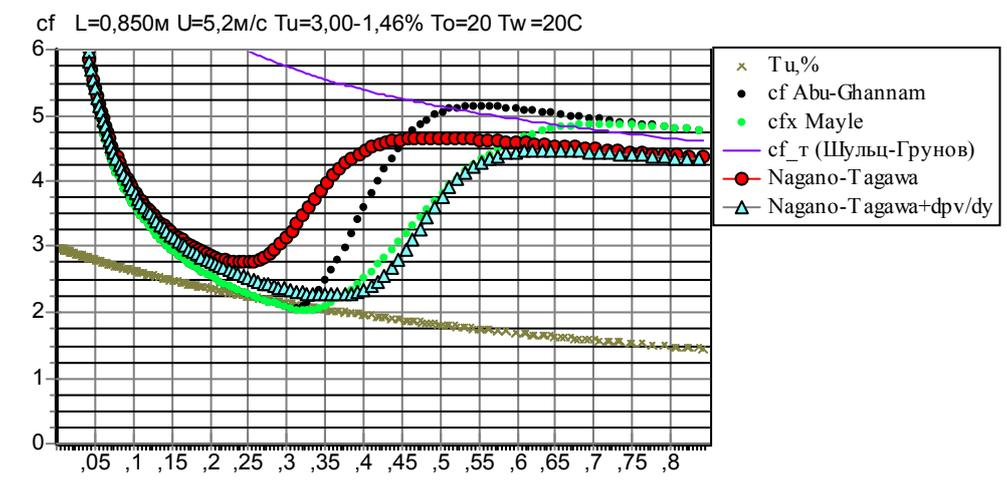
Fig. 6. Calculation of  $c_f$  friction of the laminar-turbulent transition on the plate
