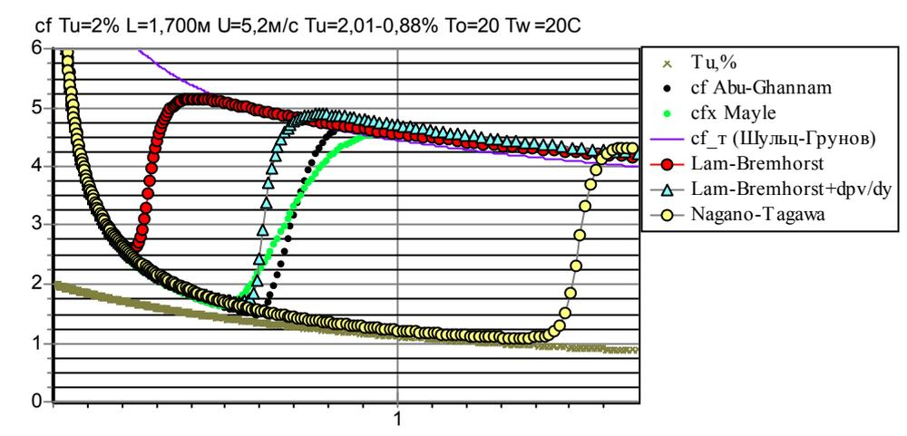
Fig. 5. Calculation of  $c_f$  friction of the laminar-turbulent transition on the plate
