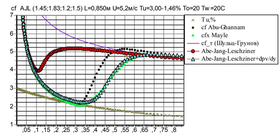
**Fig. 7.** Calculation of  $c_f$  friction of the laminar-turbulent transition on the plate
