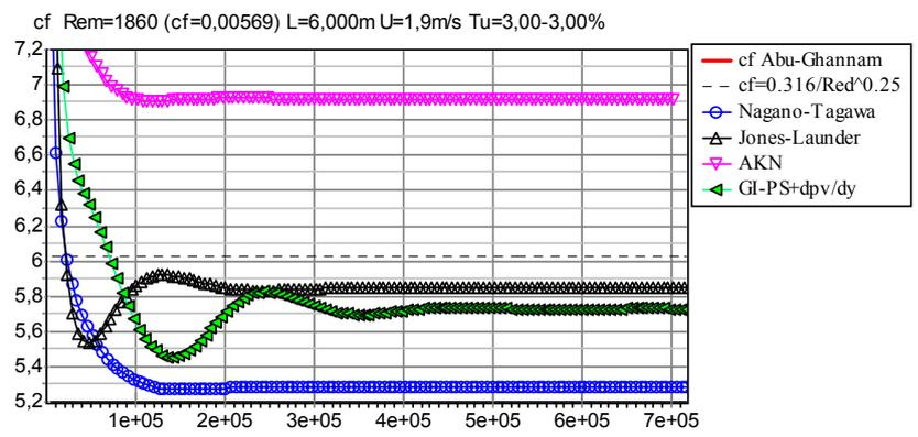
**Fig. 2.** Calculation of  $c_f$  friction in the channel (bottom axis –  $Re$  on the axial coordinate)
