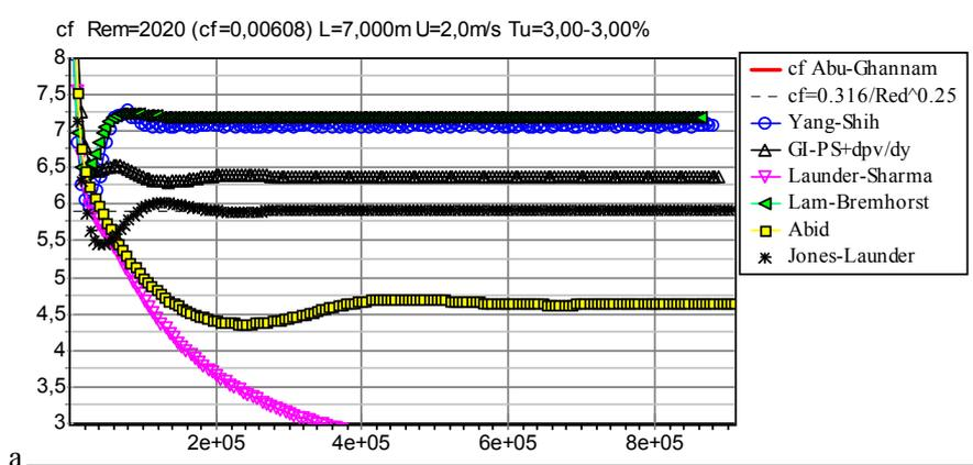
**Fig. 4.** Calculation of  $c_f$  friction (on Launder-Sharma model – degeneration into the laminar flow)
