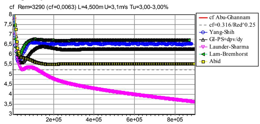
**Fig. 3.** Calculation of  $c_f$  friction (on Launder-Sharma model – degeneration into the laminar flow)
