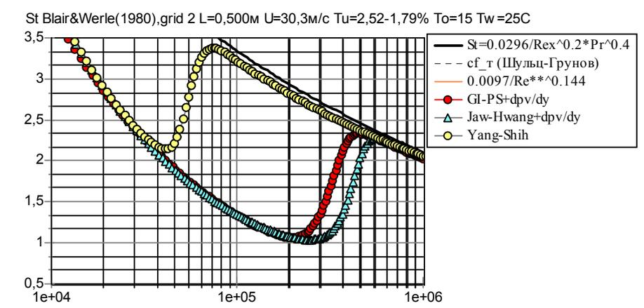
**Fig. 8.** Calculation of  $c_f$  friction of the laminar-turbulent transition on the plate
