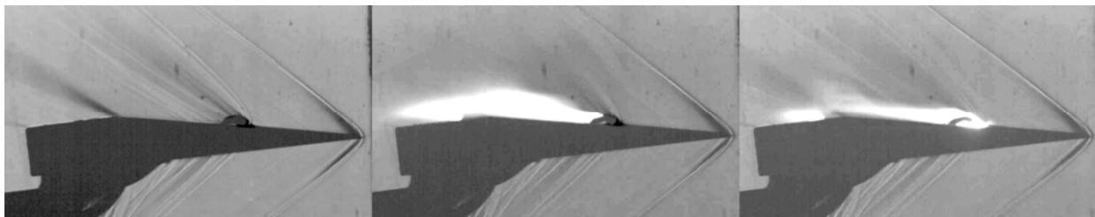
**Fig. 9. Development of the sliding discharge on the conducting surface in supersonic airflow. The exposition time of each photo is 100  $\mu$ s**
