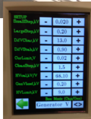
Control system for HV generators of UEWE dynamic target
