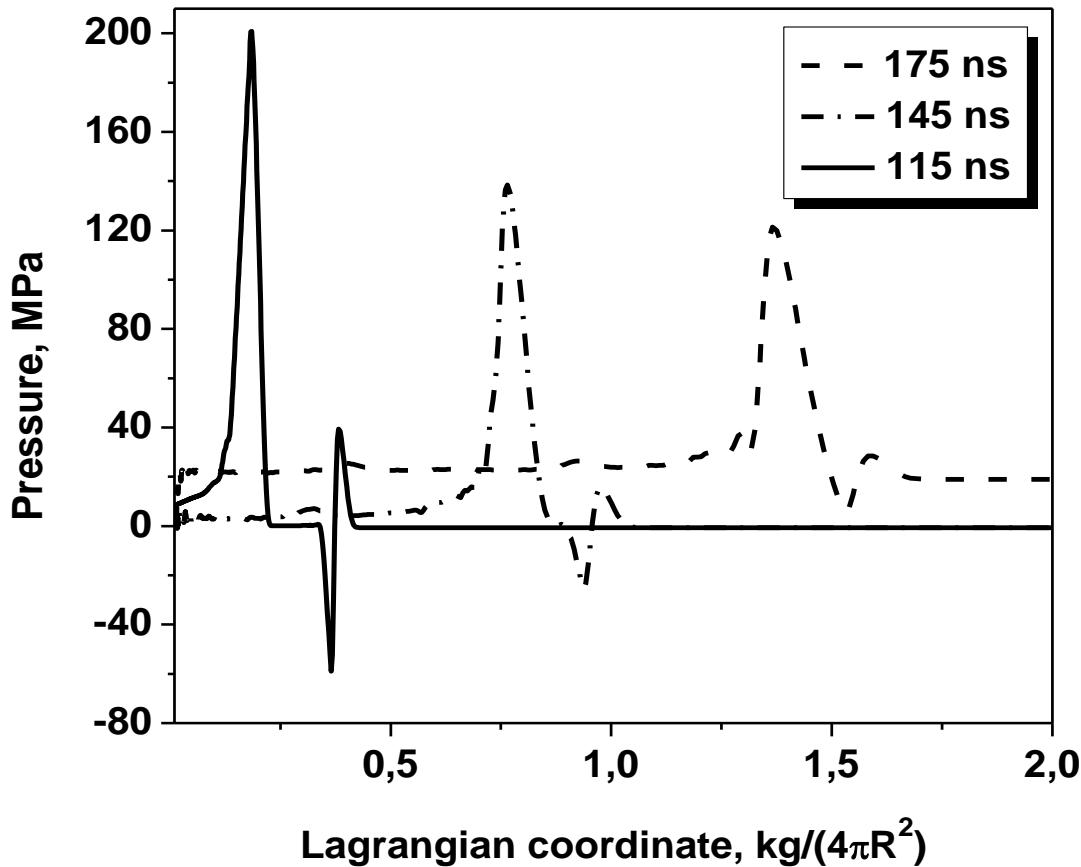
Pressure profiles in the liquid film at various times for the X-rays prepulse impact.  $R=5\text{m}$
